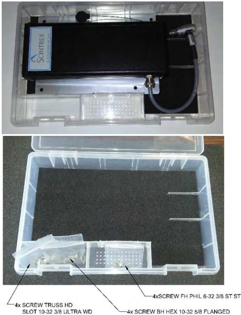
Figure 2-8 RG-1 Battery Assembly Storage Bin
