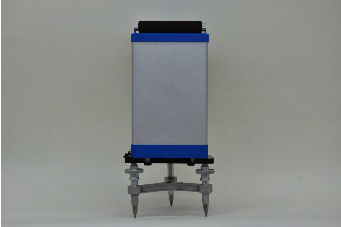
Figure 5-6 RG-1 Unit with Extended Plate Assembly, Placed on a Tripod
