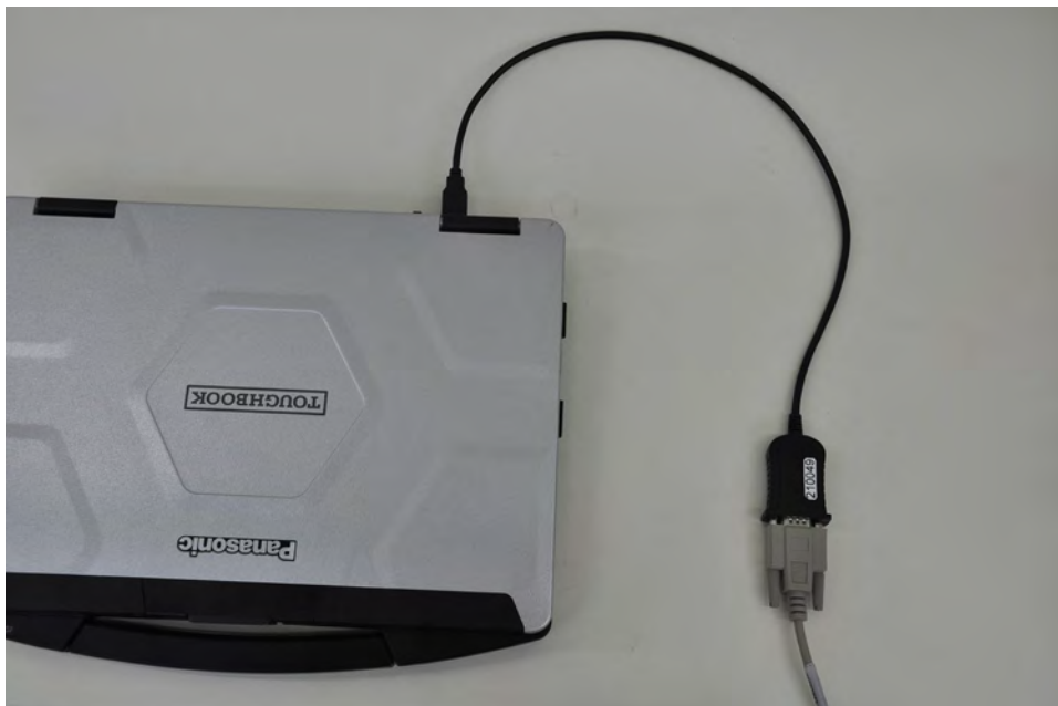
Figure 2-18 RS232 Cable connected to Laptop
