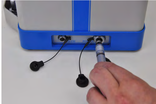
Figure 2-14 Connecting power supply to RG-1
