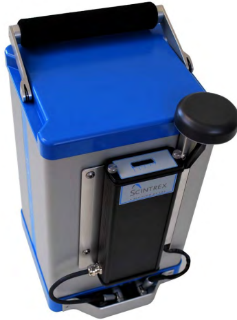
Figure 2-15 RG-1 with External Smart Battery Installed
