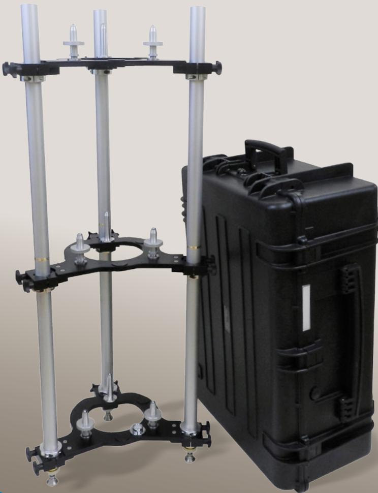
We are proud to present the latest addition to our field survey products, the TRIDENT Vertical Gravity Gradient Tripod.
