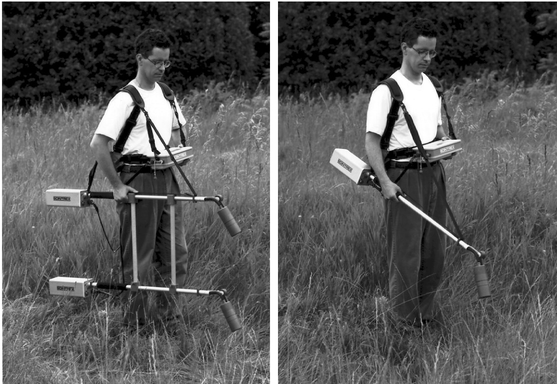
Figure 27 Surveying a test site in the Gradiometer (left) and WALKMAG (right) modes (SCINTREX SMARTMAG).
