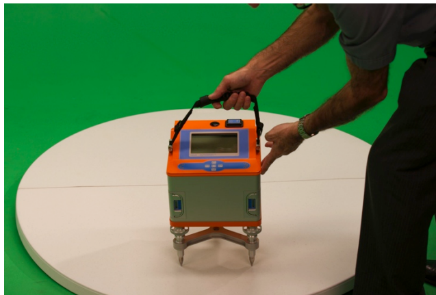
Figure 4-9 Placing the CG-6 Autograv™ on its tripod
