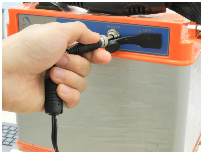
Figure 2-8 Connecting the power supply to the CG-6 Autograv™
