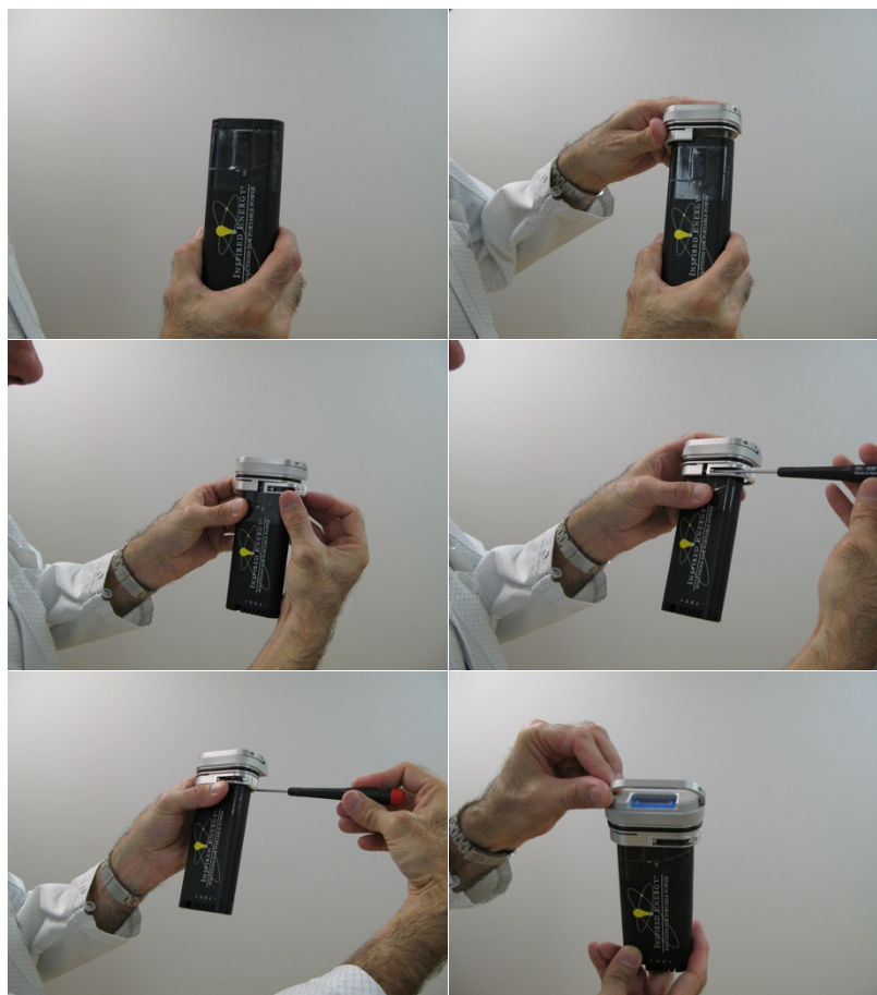
Figure 2-6 Assembling the battery packs
